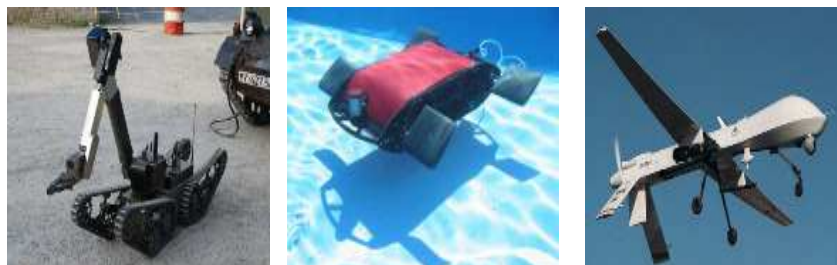
Figure 5. Terrestrial, aquatic and aerial mobile robots [Chen et al. 2009]
