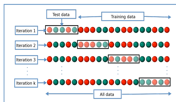
Figure 5: Cross Validation architecture [19].
