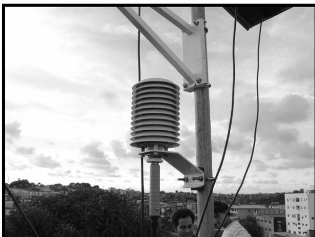
**Figura 4: Sensor HMP45C.**
