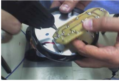
Fig. 4: Colando as placas nos spots.
